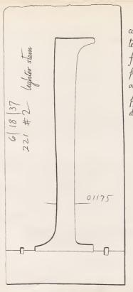
cardboard templet for making penciloutline pattern drawings these, a la French curves. You allow for the "set off of the pencil-point in cutting the templets. I used the templet method in order to keep as close as I could to the "action" of the 24 point originals.
